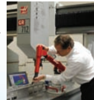
Finish inspections quickly and easily with high precision, including in-process (shown above), blueprint, incoming, first article and final inspections.
